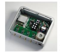
a large toroidal power transformer to maintain the instantaneous power and purity of the clock signal. The power supply for the heater and control circuits uses a separate El core transformer. By avoiding mutual interference between circuit blocks, high sound quality is achieved.
